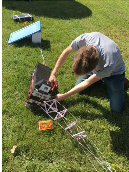
Figure 5: Insertion of MOC-SOC into P-POD during a summer launch, showing the rigging spacers on the lines below the P-POD.
