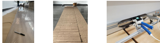
Figure 1: Balloon gores were hand-cut from a predetermined template before being sealed together
