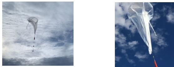
Figure 2: Zero-pressure balloons exhibiting the fill arm hanging off the side of the balloon
