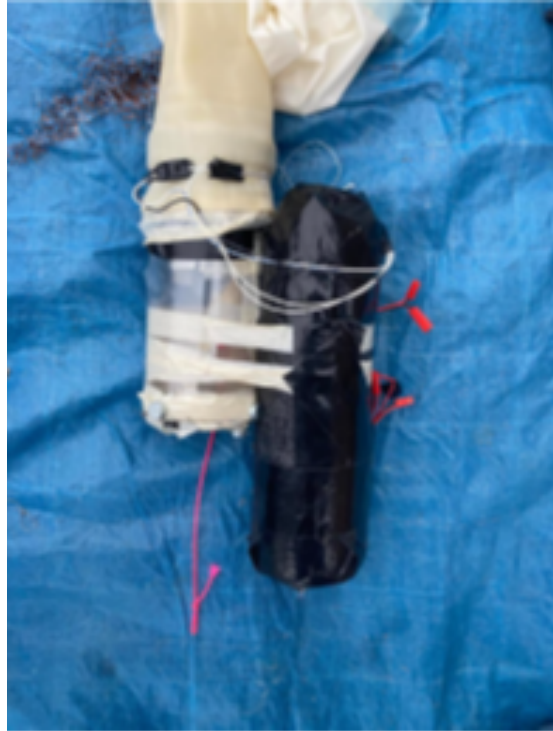
Figure 2: Photo, from Ref. 7, of Jacob Meyer's e-vent (final iteration). Avionics are inside insulated tubing (on the right) and the waist-line cut resistor is visible (in the foreground, on the left). Small permanent magnets (on the left, at the bottom) were used to strengthen the flapper seal when closed.
