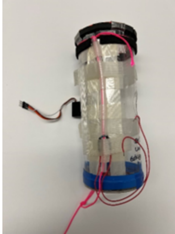
Figure 3: Photo of e-vent mechanism, with main-line lasso (and emergency cut resistor) in the foreground and servo (to be plugged into the avionics) on the left. Electrical tape is used to hold strengthening rings in place, top and bottom, and strapping tape is used to hold a tube (in the foreground) for the main line. The use of removable tape for construction makes the vent mechanism more serviceable.
