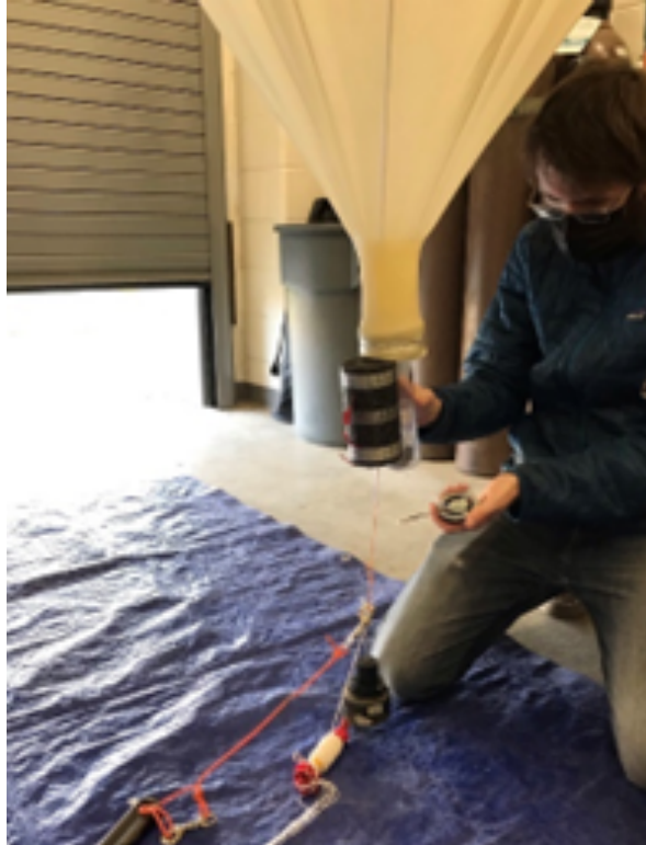
Figure 1: Photo of a HYFLITS single-use, radio-commandable vent, which only weighs about 4 oz. For a photo of this vent somewhat disassembled, with parts labeled, see Ref. 6.
