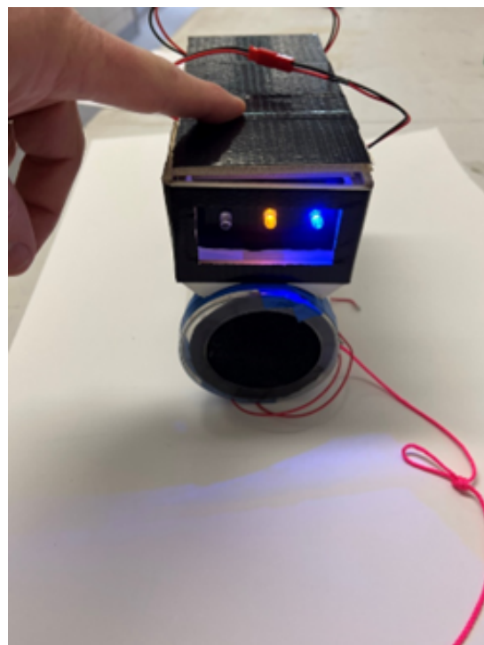
Figure 10: Avionics box on e-vent mechanism (not yet strapped down), as seen from below. The flapper is closed and the three LED indicator lights are visible.
