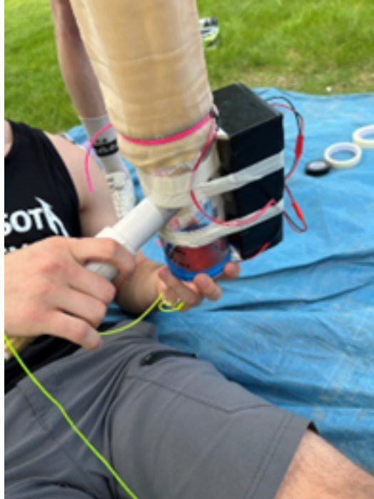
Figure 5: Inflation of a 1600 gram Hwoyee weather balloon with an e-vent installed. The avionics are in a (thin) foam-core box, rather than in a (thick) foam-insulation tubing.
