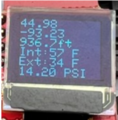
Fig. 5: Typical OLED output from a PTERODACTYL, showing gps, two temperatures, and pressure.
