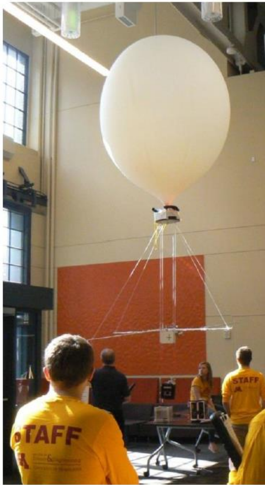
Fig. 4. A 1600-gram balloon is inflated indoors for an exhibit. Notice the parachute basket and the 8 widely-space load lines extending down to the (white) payload below and to the ends of the 3-m-long booms on the lid of the payload below. The “Goldy Gophernaut” video footage (see YouTube link in main text) came from the black box suspended below the white payload.
