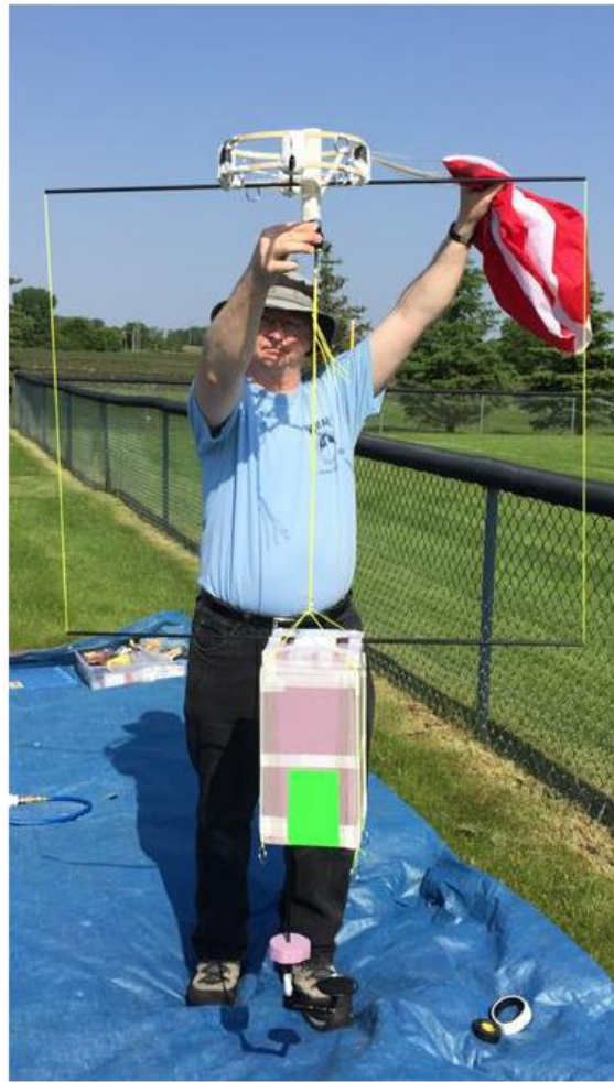
Fig. 5. Preparing a 1-D anti-rotation boom for use with a single-payload, 300-gram balloon flight. The parachute will lay in the parachute basket, made from two embroidery hoops (AKA spreader rings). The pvc tube around which the parachute basket is built, will be partially inserted into the balloon neck. The central line holds the load – 2 outer lines prevent relative rotation.
