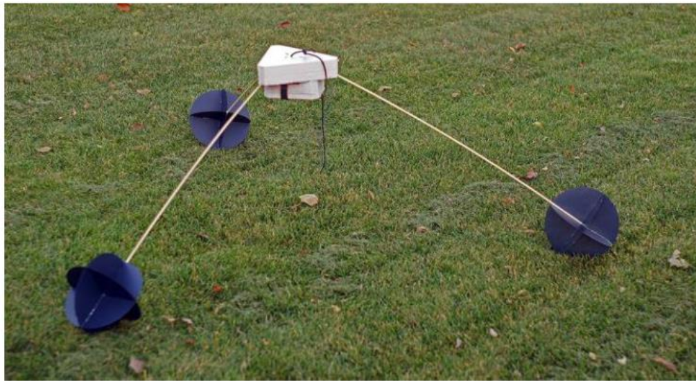
Fig. 2. Photo of Rick Brennan's built device which was flown, attached by a single line, at the bottom of a payload stack. The central part of the structure contained a video camera. Good stabilization was achieved, but only this bottom payload was stabilized.
