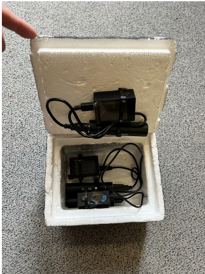
Figure 2: Three Lightdow 4000 cameras pointing up, down, and out, each with an external battery pack, in a small payload box. The total weight of this payload, once rigging is added, is only 22 oz. The total cost is less than that of a single GoPro HERO5 Session camera.
