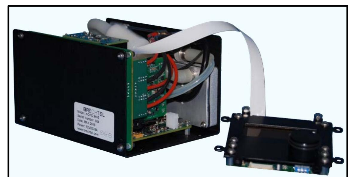
Image showing the Brechtel Miniature Optical Particle Counter (mOPC) that rapidly measures the aerosol number size distributions. The mOPC size is 9.4 x 11.9 x 15.2 cm and weight is 1.0 kg.
