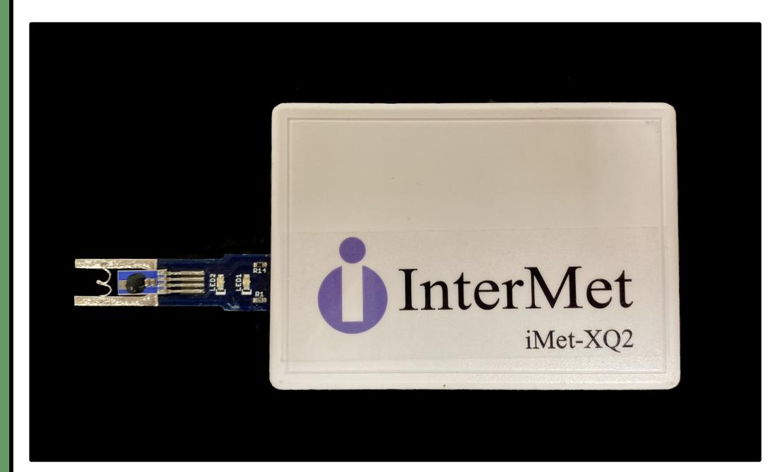
Image showing Imet-XQ2 that measure temperature, relative humidity, pressure, and GPS position. The size is 3.25 x 2.25 x 0.875 inch and weight is 60 g.
