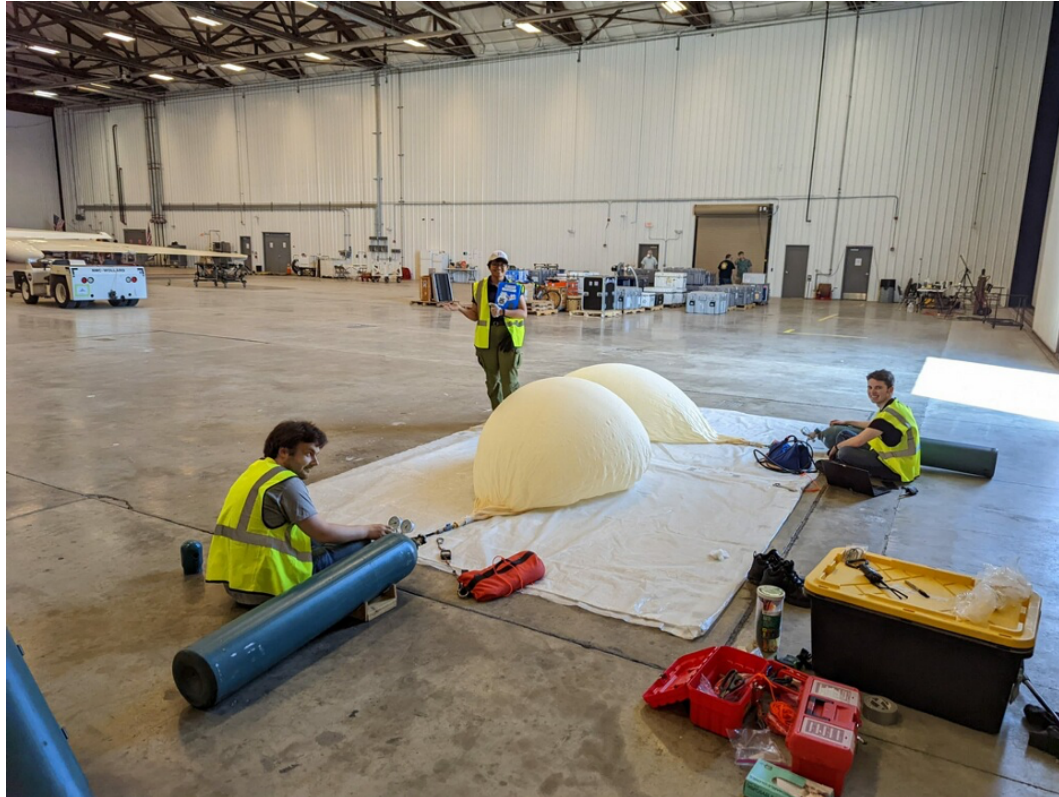
Figure 2: Simultaneous inflation of two 1600g latex balloons - the neck of each balloon is already tied to an anchoring sandbag with an inline lift measuring scale
