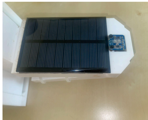
Fig. 5. Assembled solar panel and luminosity sensor in HAB@VT laboratory.
