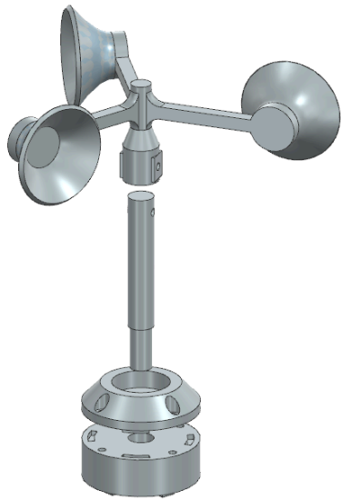
Fig. 11. Exploded view of how the anemometer is assembled.
