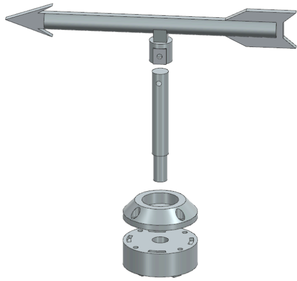
Fig. 12. Exploded view of how the wind vane is assembled.
