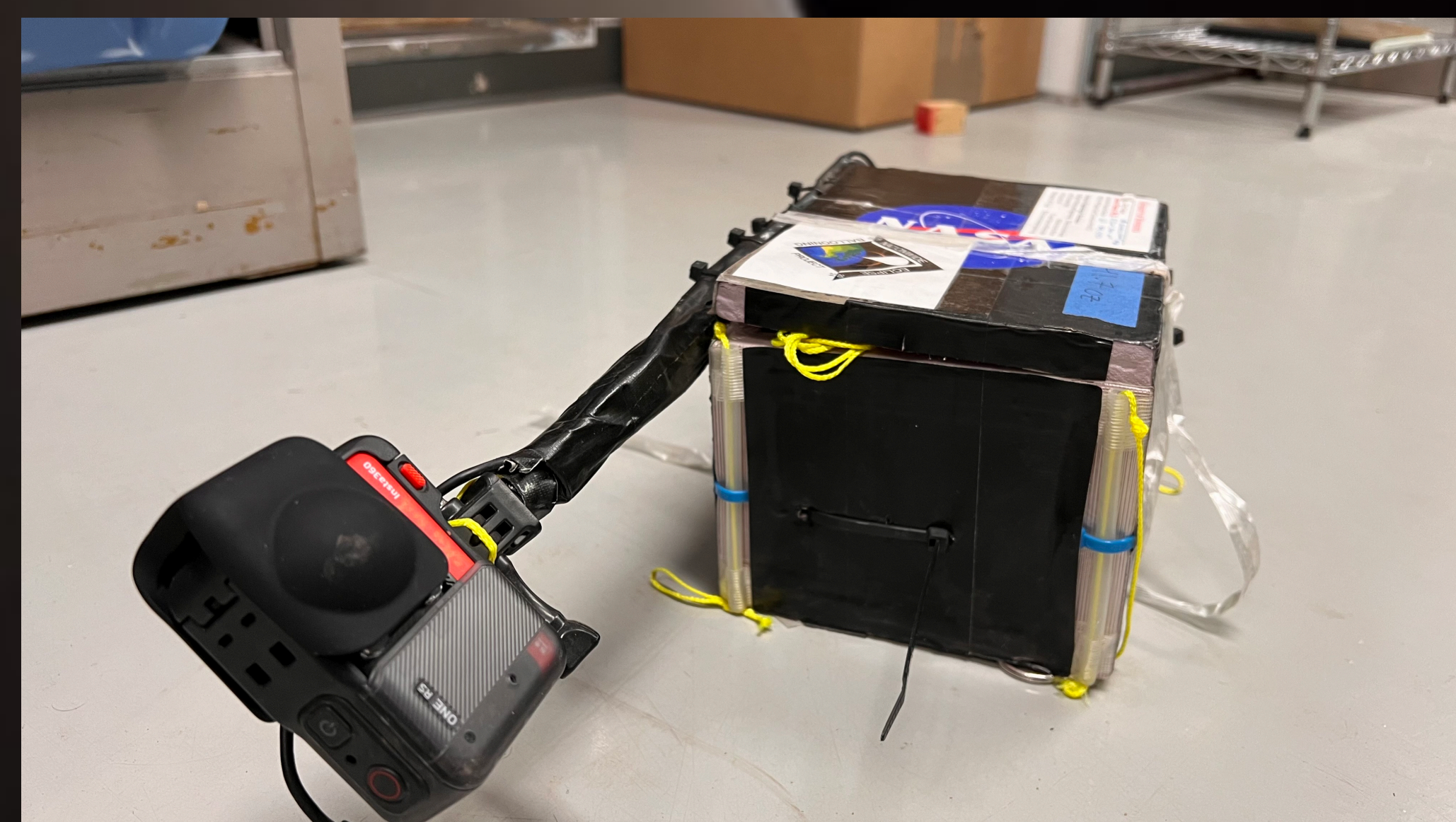
Image 1, Insta360 one RS attached to payload
