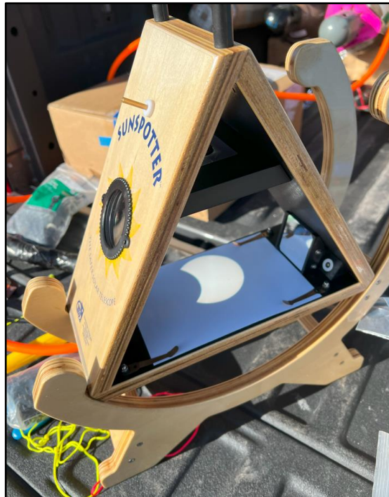
Fig. 2. A Sunspotter solar telescope projecting an image of the beginning of the annular eclipse in 2023.
