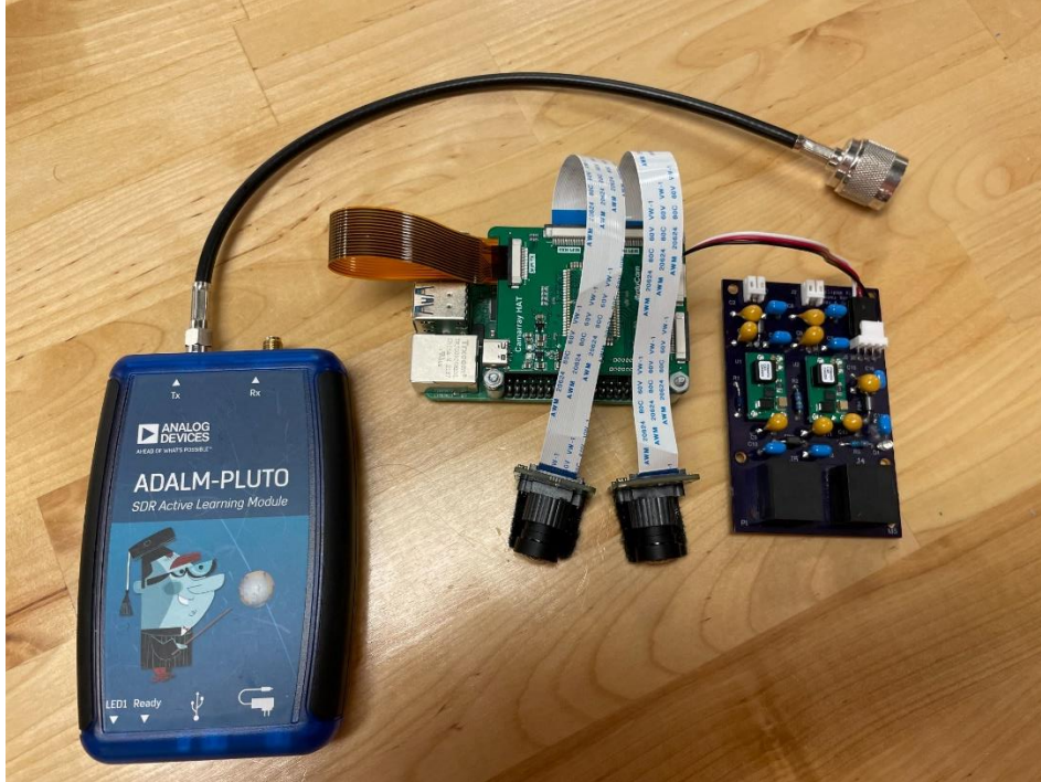
Fig. 3. The hardware configuration if the PlutoSDR board is used. This specific setup relies on a Power-Over-Ethernet (POE) custom board by the HAB students at the University of Montana to power a Raspberry Pi 4B CamArray hat for multi-camera video feeds.
