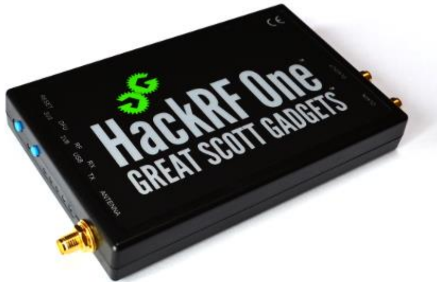
Fig. 4. A photograph of the replacement SDR board, the HackRF One by Great Scott Gadgets. This new device has a wider range of standard operation starting as low as 1 MHz and as high as 6 GHz, a much higher sample rate capacity of 20 MSPS. This device has a slightly higher power draw than the PlutoSDR because of these improvements, [8]
