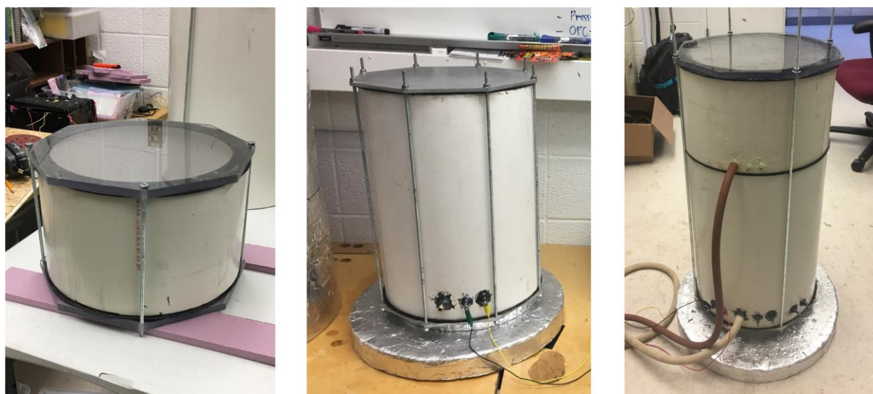
Fig. 1: The three different length-configurations of the thermal-vac chamber.
