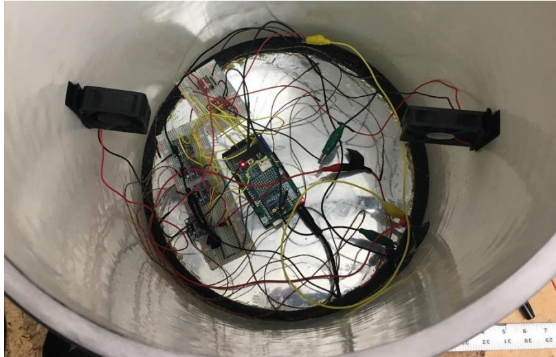
Fig. 3: The Arduino Mega microcontroller system in the bottom of the thermal-vac chamber for monitoring internal pressure plus temperature at four independent locations. Two fans are attached to the chamber walls. The Arduino Mega is powered through one pair of electrical feed-throughs (lower right). Additional electrical feed-throughs can be used to power items under test, if desired, to limit the number of batteries expended during testing (though payloads are often tested with batteries in place, if battery performance is one of the things being tested).
