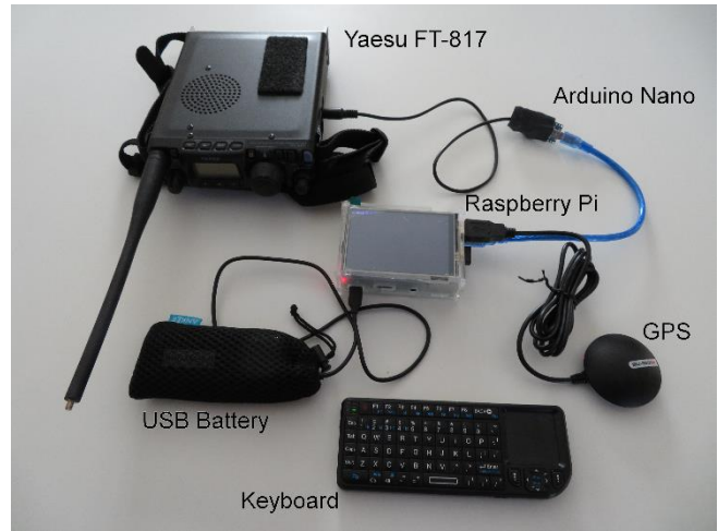
Figure 4. Implementation using an Arduino Nano and Yaesu FT-817 radio
