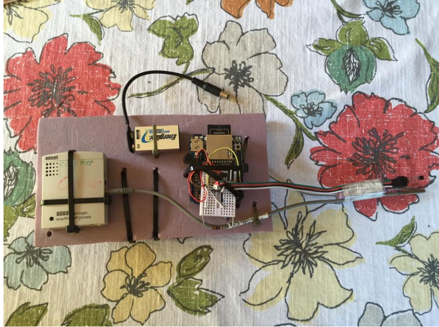
Fig. 4a Triple-temperature logger. HOBOTemp and Arduino loggers visible; Neulog modules on underside.
