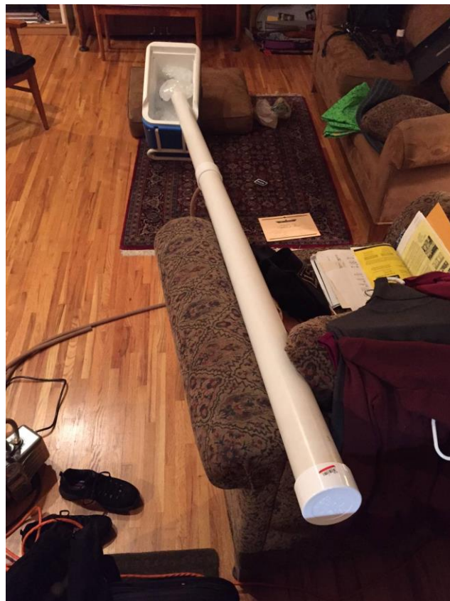
Fig. 5b The 3-inch diameter PVC pipe used for the reduced-pressure test. The pipe was evacuated through the vacuum hose attached to the central coupler. The far end of the pipe was kept at ice temperature.
