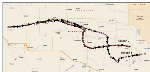
Figure 1: Balloon Trajectories. Balloon 1 reached 102,500 feet and Balloon 2 reached 102,050 feet. The student chase vehicle tracked Balloon 2.
