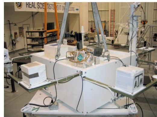
Figure 2. Top view of the HASP system showing location of the small payloads on booms and large payloads on top of the main structure.
