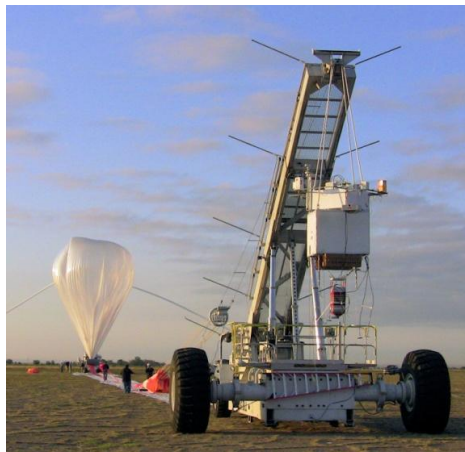
Figure 5. Balloon inflation is underway while HASP is performing a final check-out just prior to launch.
