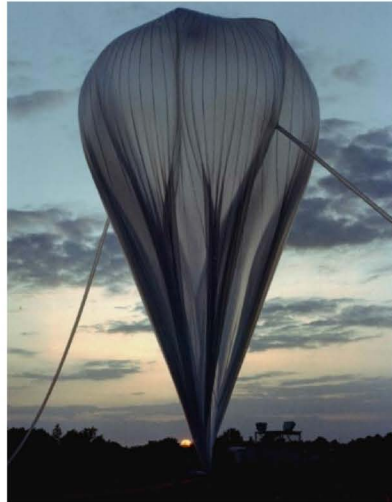
Figure 2: A Zero-Pressure Balloon Operated by the NASA Goddard Space Flight Center [16]
