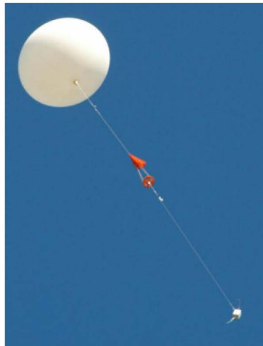
Figure 1: A Latex Balloon & Payload Train [14]
