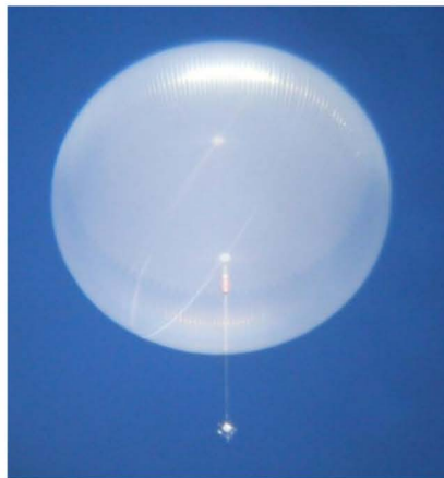
Figure 3: A Super-Pressure Balloon [19]
