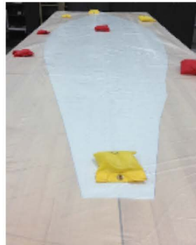
Figure 5. Two layers of sheeting over gore pattern.
