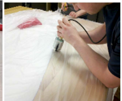
Figure 6. Final gores being sealed.
