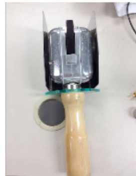
Figure 3. New roller for seam sealing.
