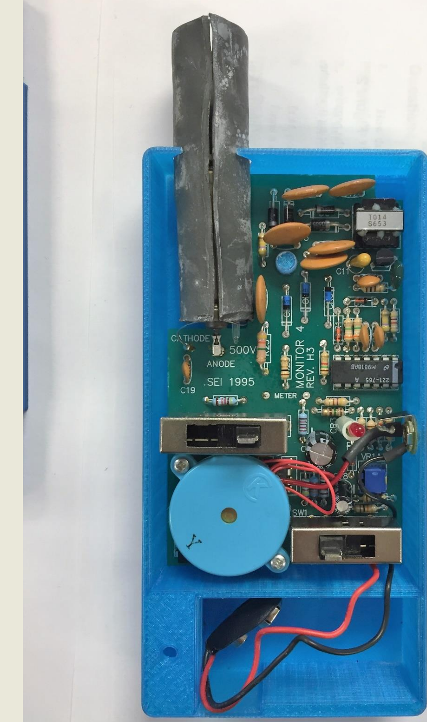
Figure 2: The lead collimated Geiger counter with adjusted peripheral detection range
