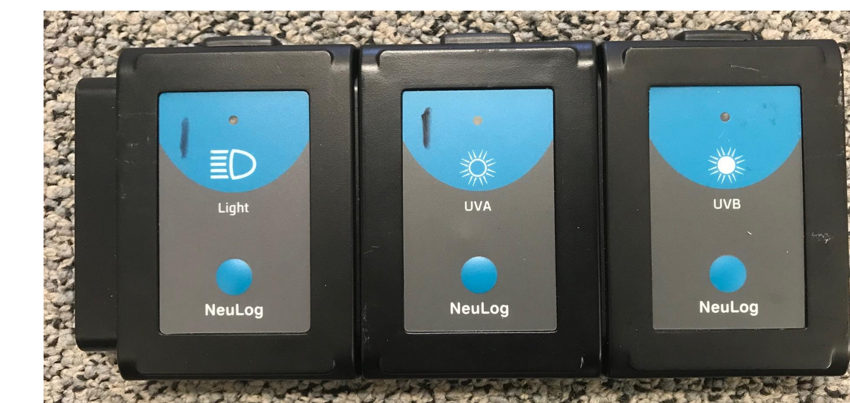
Figure 5: Chain of 3 light-sensing Neulog modules: visible to ultraviolet.
