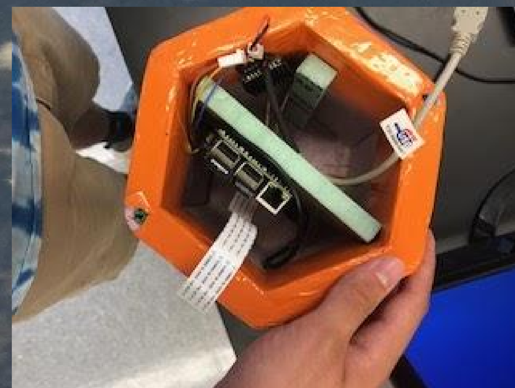
RFD payload that was redesigned to be more compact and waterproof.
