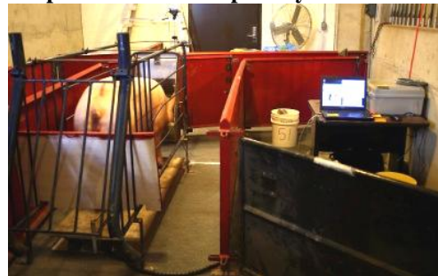
Figure 2. Embedded Prototype Embedded Micro-computer-based force plate system.
