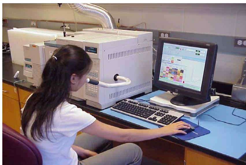
Figure 2. Simultaneous chemical and olfactory analysis of odor and VOCs emitted from poultry manure using GC-MS-O.
