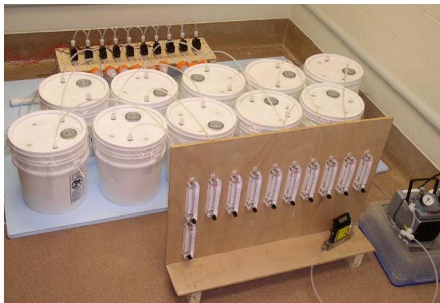
Figure 1. Laboratory set up for testing of the effects of zeolite treatments on odor and VOCs emissions from poultry manure.
