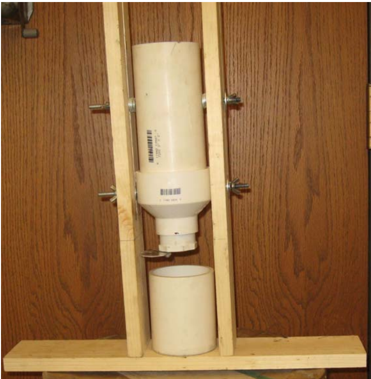
Figure 2. Fabricated device for measuring bulk density of feedstuffs and diets.
