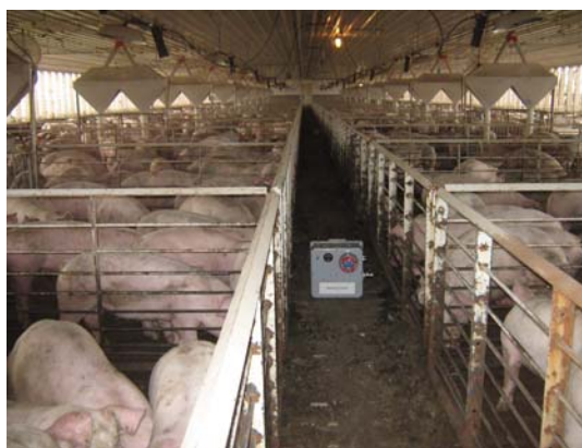
Figure 1. The previously developed wireless H 2 S detection system deployed in a swine facility prior to slurry agitation and removal.
