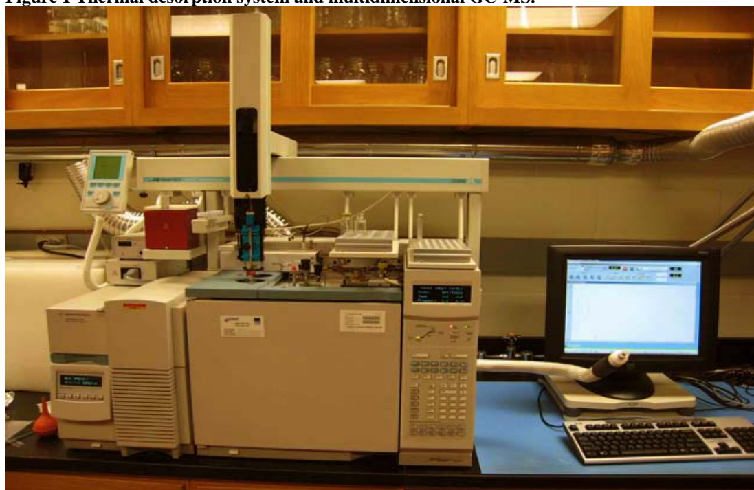
Figure 1 Thermal desorption system and multidimensional GC-MS.
