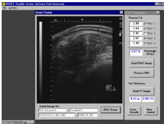
Screen 10. Cross-sectional image after fat thickness has been measured (0.43 in) at the 3/4 position on the 1. dorsi muscle and converted to yield grade (2.88).
