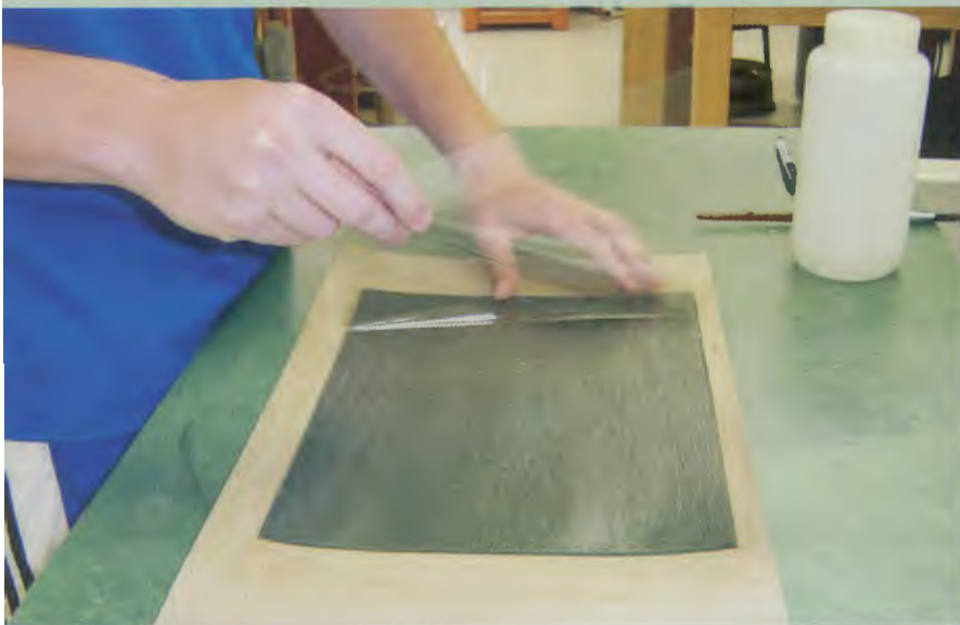
Andrew Hoppmann, ISU student employee in Preservation, demonstrates the preparation of a Mylar sheet support for lens tissue used in backing fragile documents.
