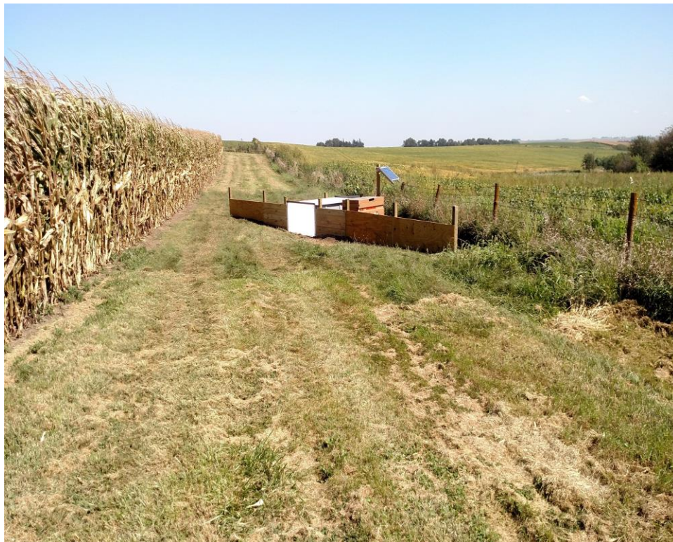
Figure 2. Flume structure at the control site, Armstrong Research Farm, Lewis, Iowa.
