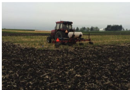
Figure 1. Side-dresser used for applying liquid UAN to Miscanthus plots prior to planting.
