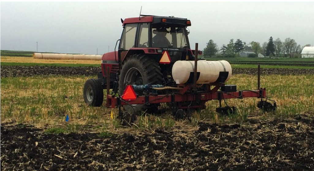
Figure 1. Side-dresser used for applying liquid UAN to Miscanthus plots prior to planting.
