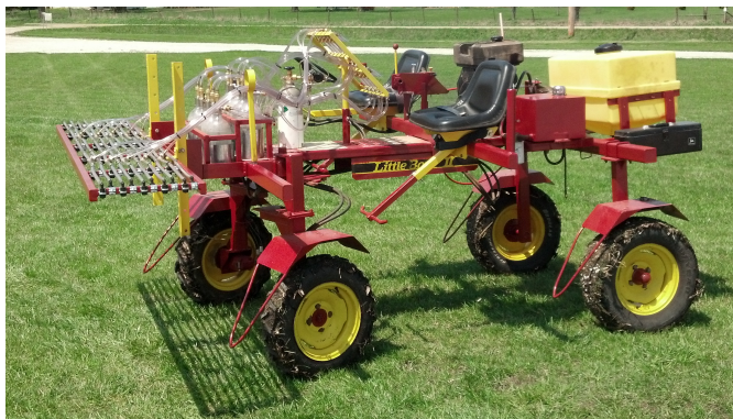
Figure 2. Self-propelled research sprayer built by Iowa State personnel.
