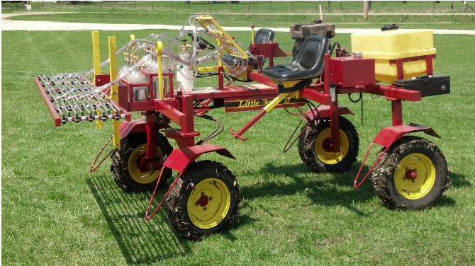
Figure 2. Self-propelled research sprayer built by Iowa State personnel.
