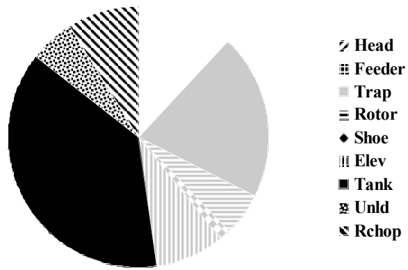
Figure 1. Relative amounts of soybeans and other biomaterial collected from cleaning various areas of a rotary-type combine.
