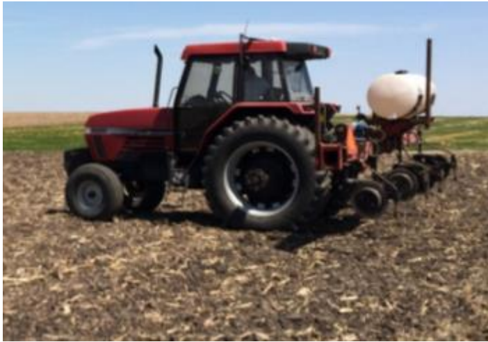
Figure 1. Side-dresser used for applying liquid UAN to M. × giganteus plots prior to planting.
