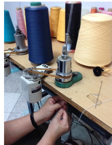
Figure 1: Knitting with six-needle cord knitting machine
