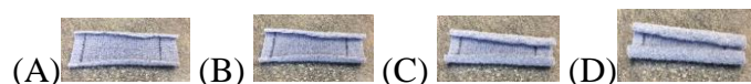
Figure 1. Screen shots from a video recording showing responsiveness of pattern #10 in wool yarn: (A) 1 second after applied moisture, (B) 5 seconds after applied moisture, (C) 10 seconds after applied moisture, and (D) 15 seconds after applied moisture.
