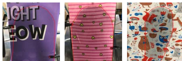
Figure 3: Surface wetting of the fabrics after hot splash. Fabrics from left to right are p/ jersey, p/fleece, and C/M interlock
