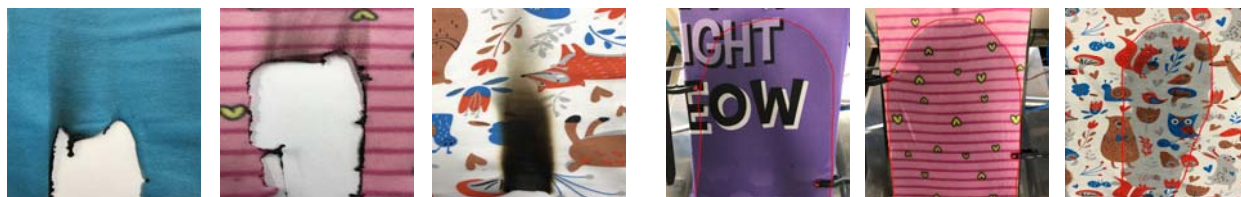
Figure 1: Fabric response in vertical flammability tester. Fabrics from left to right are p/ jersey, p/fleece, and cotton/modacrylic (C/M) interlock.
