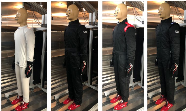
Figure 2. From left to right: Base layers, SFI-1 Suit, SFI-5 Suit, SFI-20 Suit. Each suit was tested with and without base layers.
