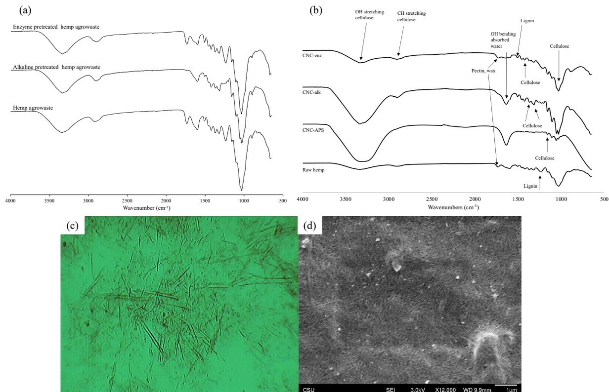
**Figure 1.** (a) ATR-FTIR spectra of alkaline and enzyme pretreated hemp agrowaste, (b) ATR-FTIR spectra of prepared CNCs, (c) OM and (d) SEM images of CNC-alk
