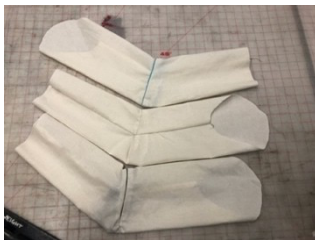
Figure 2: Sleeve prototype development for neutral posture with resistance stretch on elbow joint.
