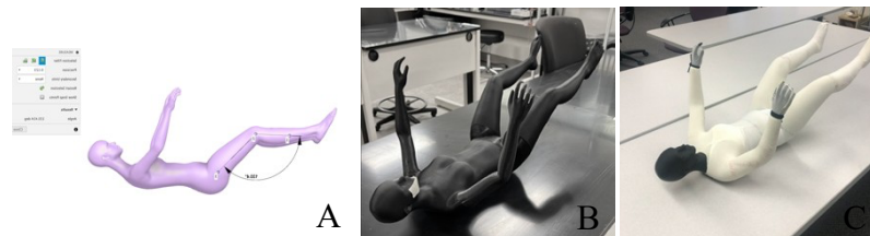
Figure 1: A. Avatar in neutral body position in CLO 3D, B. 3D printed half scale avatar, C. Foam covered pinnable avatar.
