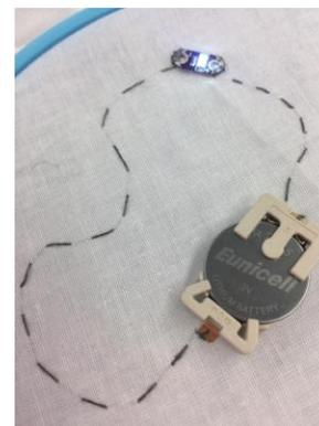
Figure 1 Electronic components in a series circuit
