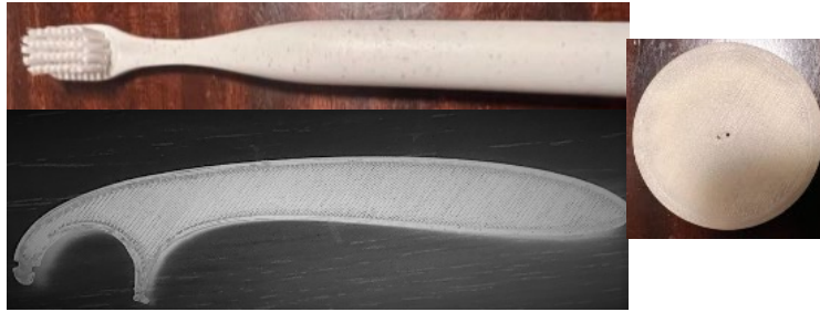
Fig. 4 3D printed consumer products with PLA-cotton composite.
