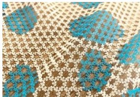
Figure 1. The ripple auxetic structure textile
