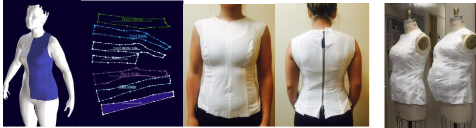
Figure 1. 3D flatten tool and 2D patterns in Optitex, test garment on the body, custom dress forms
