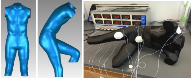
Figure 1. Digital/3D printed forms in standing and cycling poses, and measuring pressure
