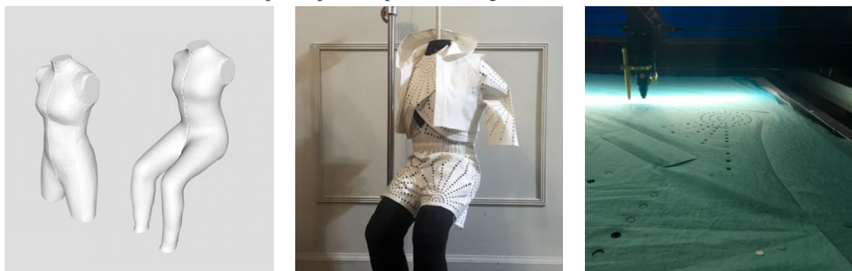
Figure 1. Left: Processed standing and sitting 3D body scans ready to be made into half-scale dress forms. Middle: Draping garments on seated position form to check fit and utility. Right: Laser cutting fashion fabric
