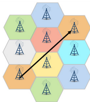
Figure 2. Frequency reuse through geographical separation (Qualcomm, 2014).
